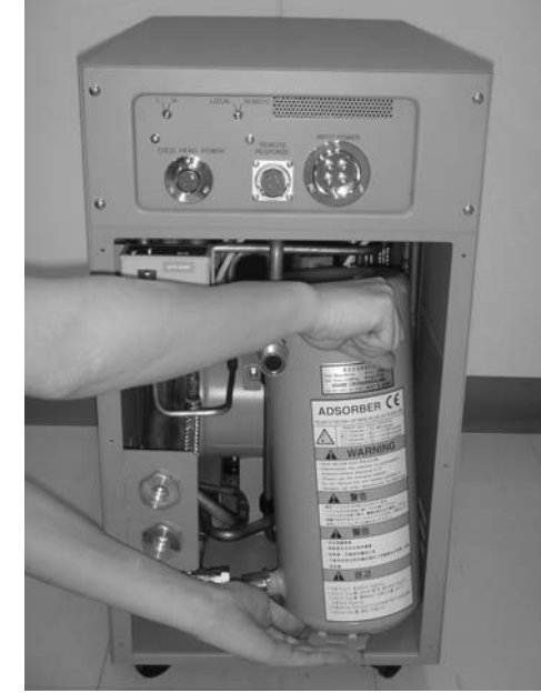
④ Draw the adsorber out of the compressor unit.
