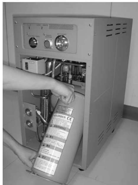
※ Draw the adsorber out of the compressor unit by learning it. (Do not touch the piping.)
