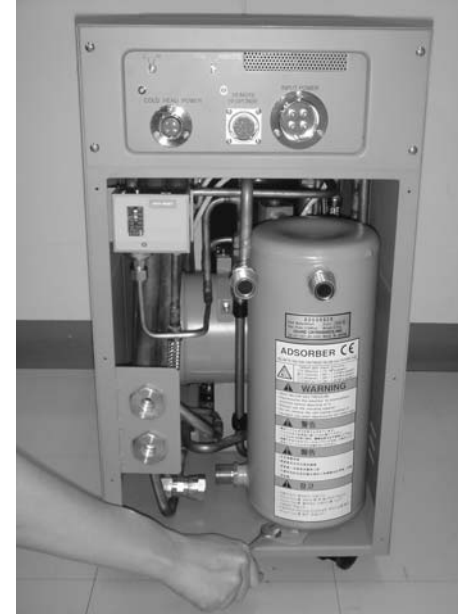
③ Remove the adsorber mounting bolt.
