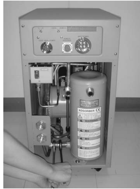
② Disconnect the flexible hose from the adsorber inlet.
