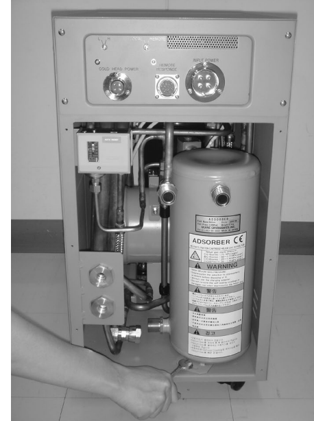
③ Remove the adsorber mounting bolt.
