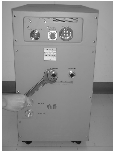
① Remove the jam nuts. Remove the rear panel from the compressor unit by unscrewing 7 screws.
