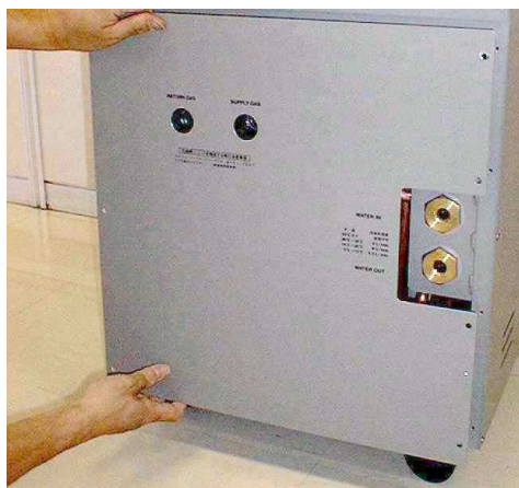
Figure 6-1 Remove Two Nuts from the Helium Gas Connectors
