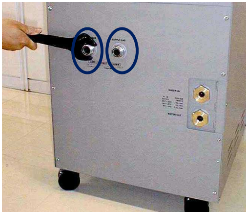
Figure 6-1 Remove Two Nuts from the Helium Gas Connectors
