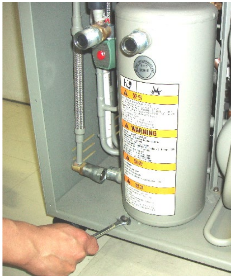
Figure 7-6 Remove adsorber mounting bolt (left)
