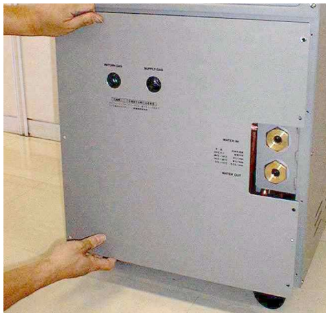
Figure 7-3 Remove the rear panel (left)
