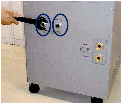
Figure 7-1 Remove two nuts from the helium gas connectors
