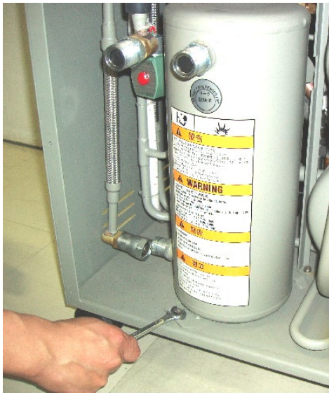
Figure 7-6 Remove adsorber mounting bolt
