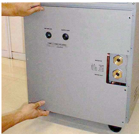
Figure 7-3 Remove the rear panel
