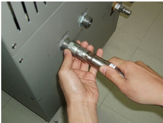
Figure 4-2 Fasten with hands first
