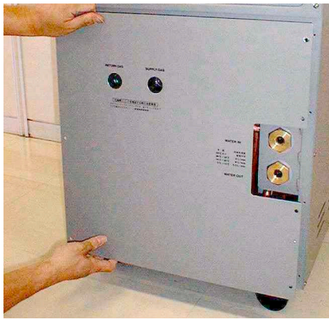
Figure 7-3 Remove the rear panel
