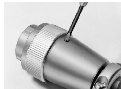
Figure 4-12 Fix with set screw
