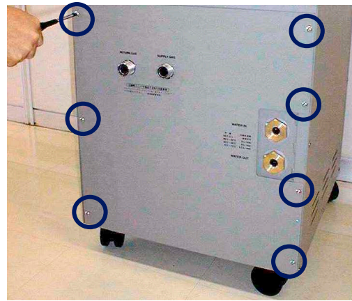
Figure 7-2 Remove seven screws from the rear panel
