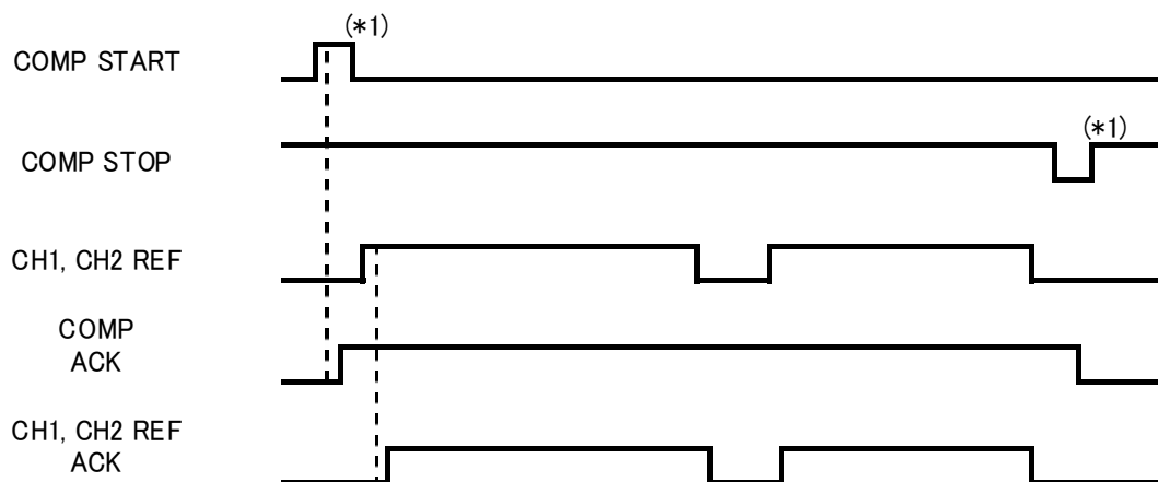
Figure 2-6 Timing chart for Alternate operating mode with two refrigerators
