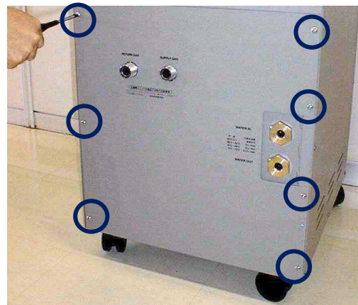
Figure 7-2 Remove all seven screws from the rear panel
