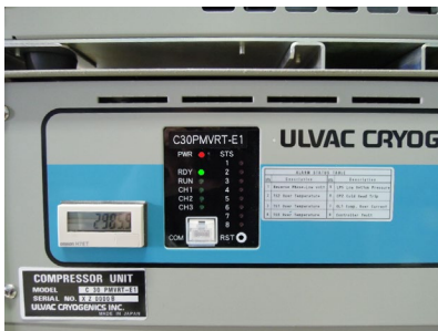
Figure 5-2 Ready for operation
