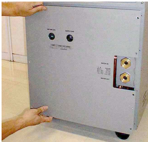
Figure 7-3 Remove the rear panel
