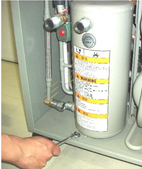
Figure 7-6 Remove adsorber mounting bolt
