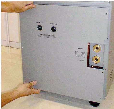
Figure 7-3 Remove the rear panel
