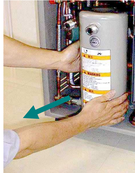
Figure 7-7 Slide adsorber outward
