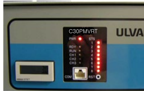
Figure 5-4 Reversed phase or open phase
