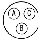
This is the socket side insert, as seen from the pins at front of connector.
