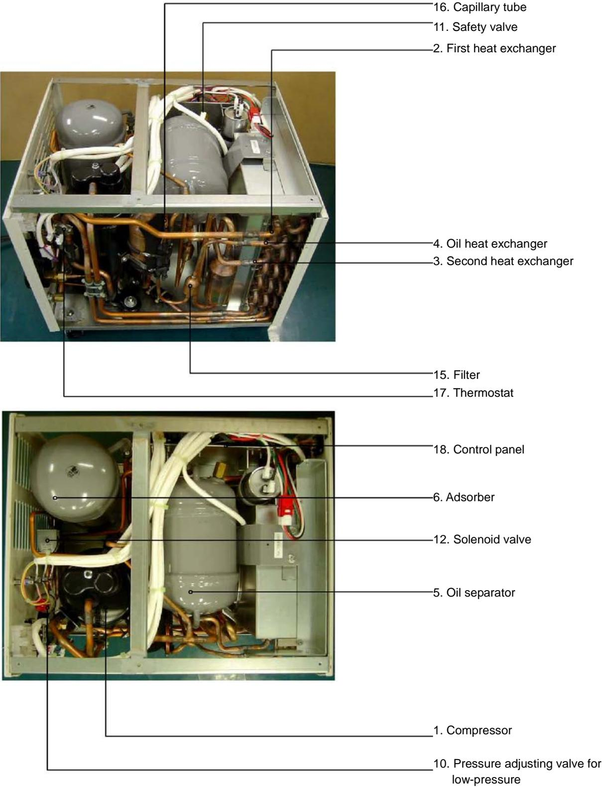
**Figure 3-3 SA112-C Interior Components**
