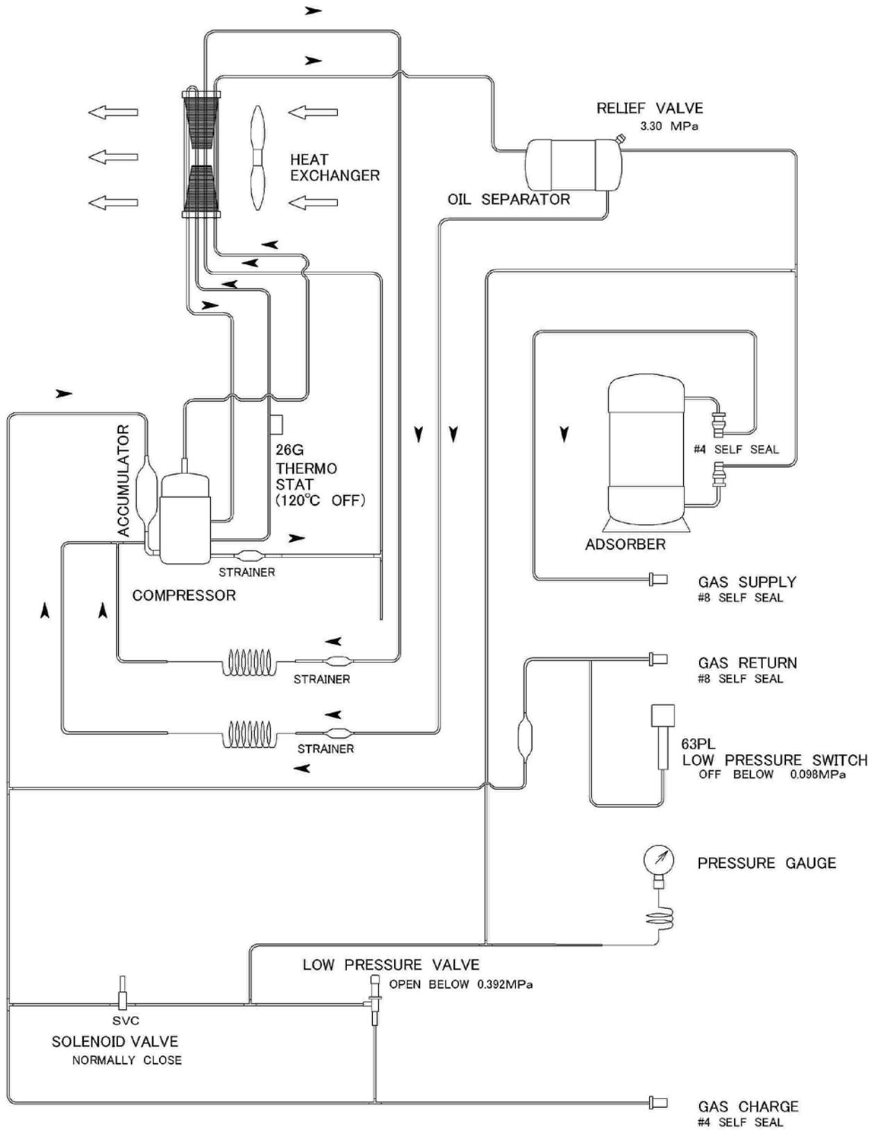
**Figure 3-2 Refrigerant Circuit Diagram**
